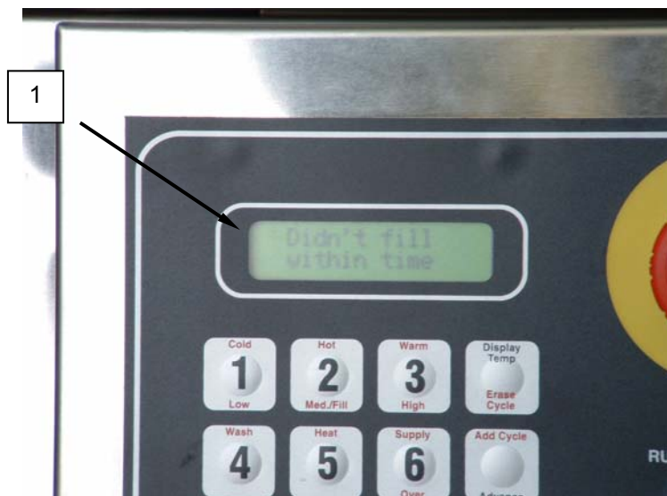
Figure 1. Didn't fill within time Error on Washer Display.
