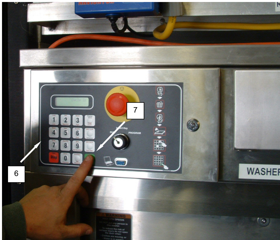
Figure 9. Nanofilter Cleaning Procedure – Start Cycle 59 on Washers.
