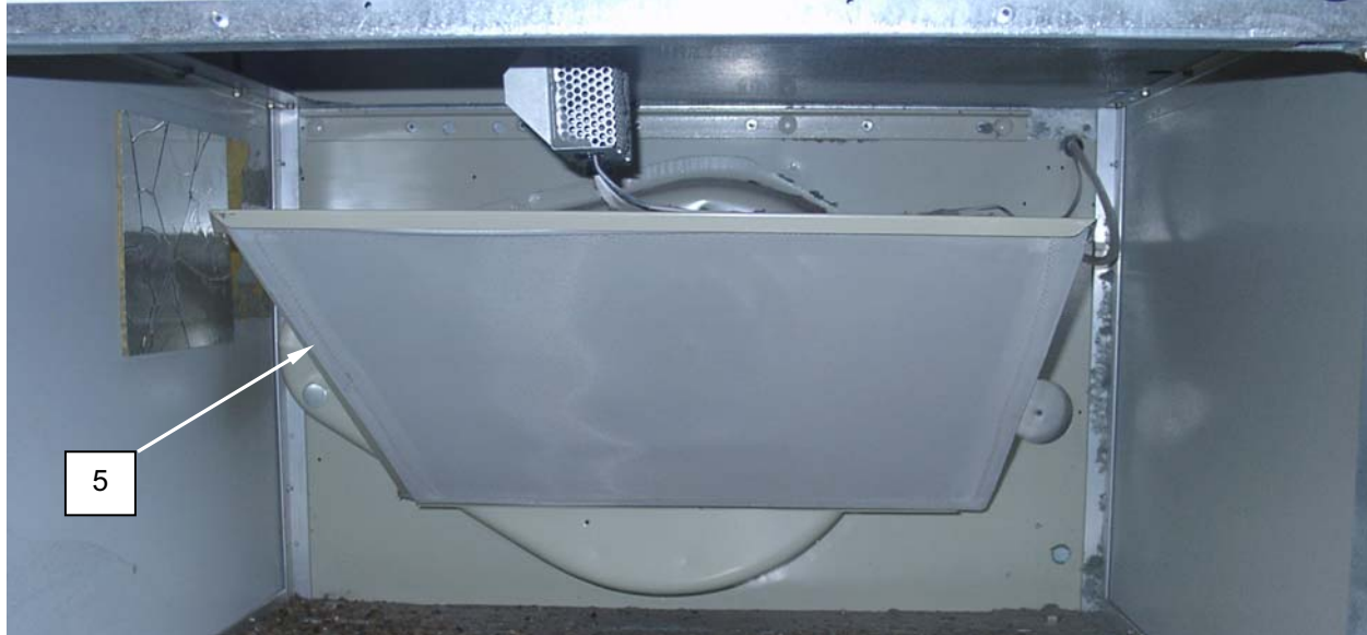
Figure 2. Clean Dryer Lint Screens.
