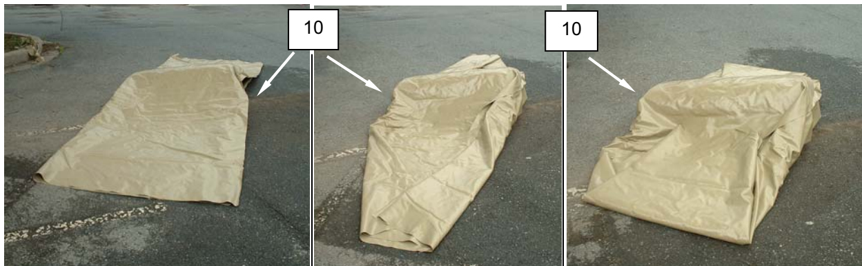
Figure 8. Prepare the 3000 Supply Water Tank for Movement.
