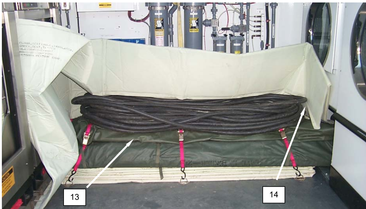
Figure 12. Placing the Cables for Full Packout.
