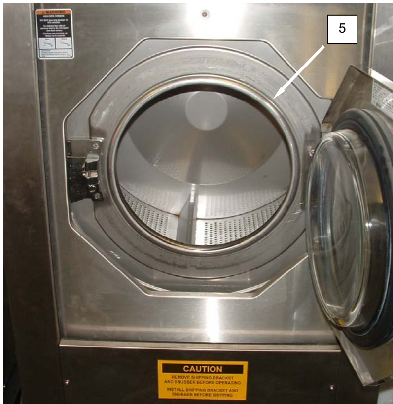
Figure 5. Nanofilter Cleaning Procedure – Add Chemical to Washer Drum.
