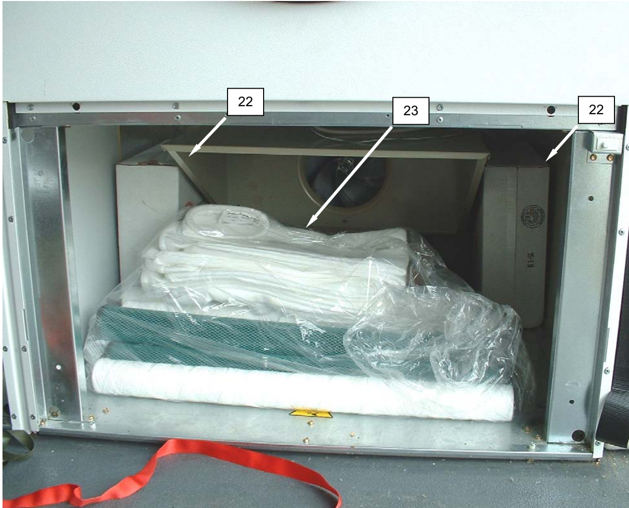
Figure 18. Placing the Pond Heater and the Filter Elements.
