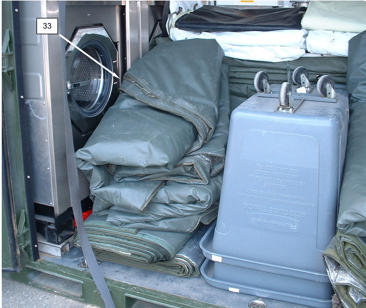
Figure 30. Place Second Set of Water Tank Insulation.
