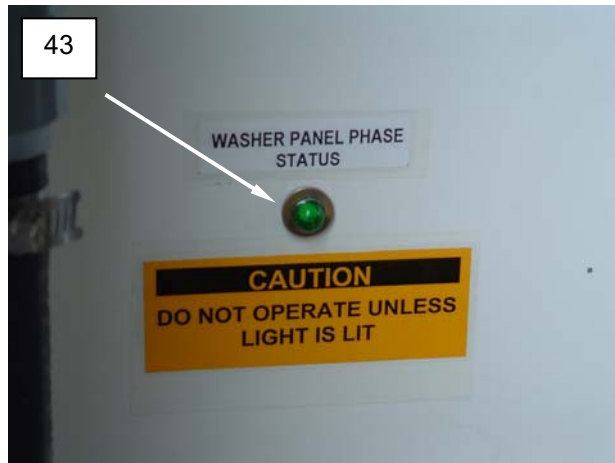
Figure 12. Check Phase Indicators.
