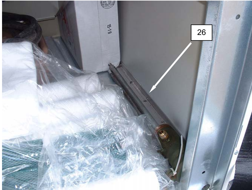
Figure 21. Fuel Can Adapter between Filters and the Dryer Cabinet.
