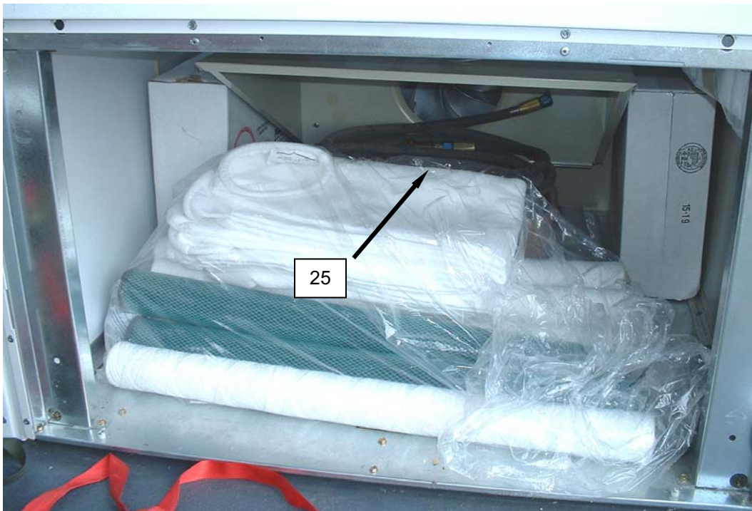
Figure 20. Fuel Hoses on Top of Fuel Can.
