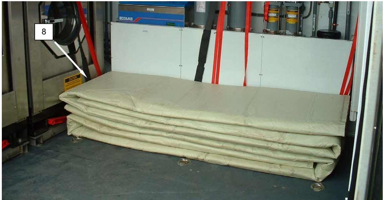
Figure 7. Folded TEMPER Flooring.
