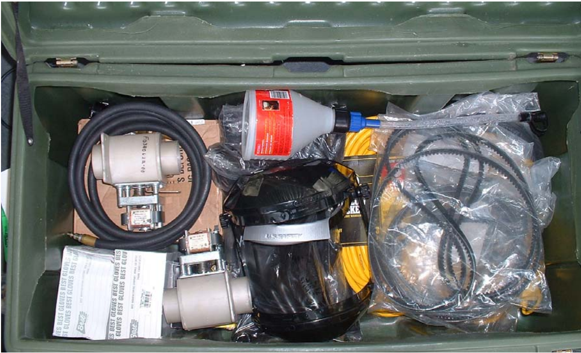
Figure 4. Packing Spare Belts, Hoses, and Valves.
