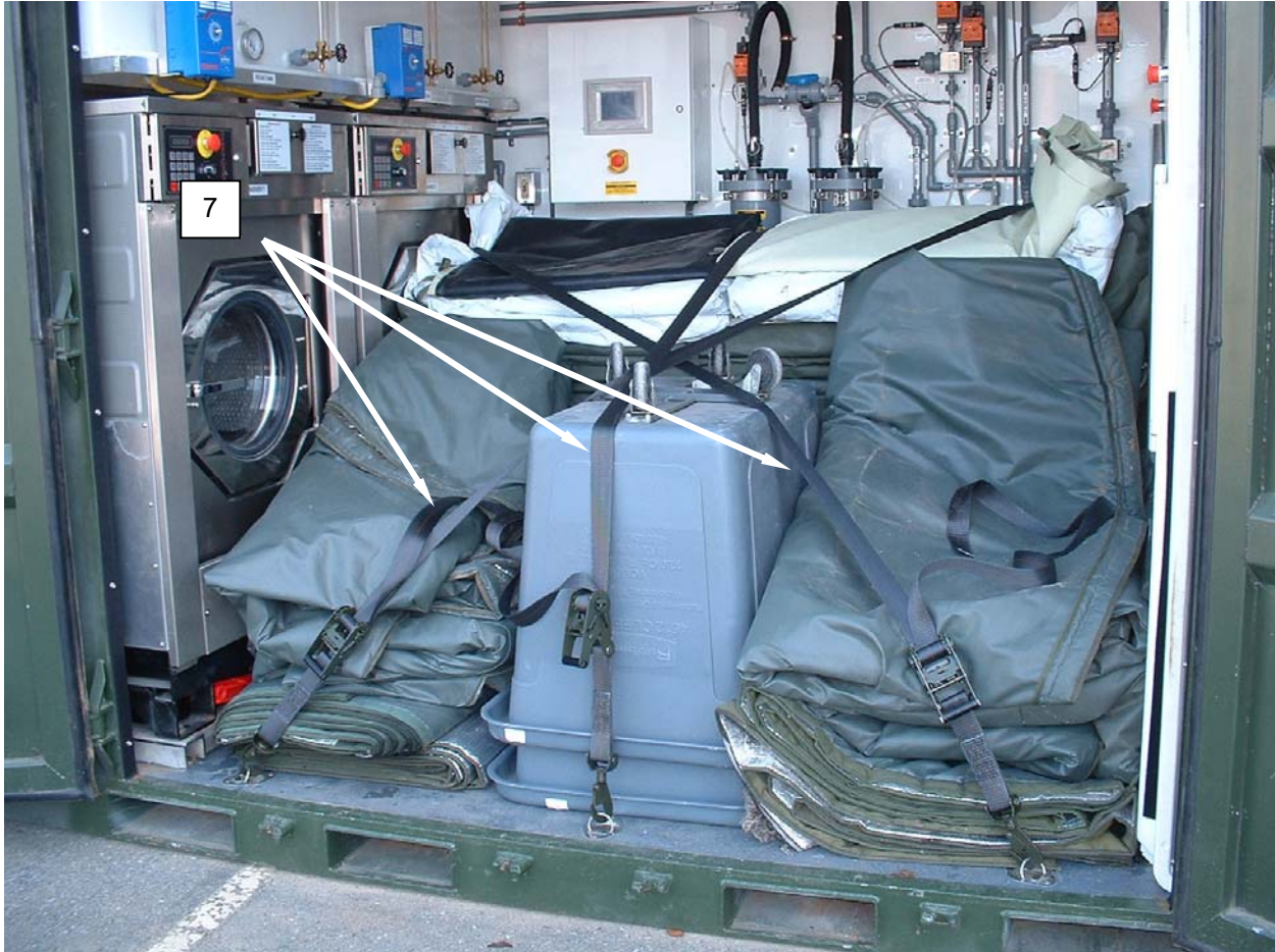
Figure 31. Secure Center Strap.
