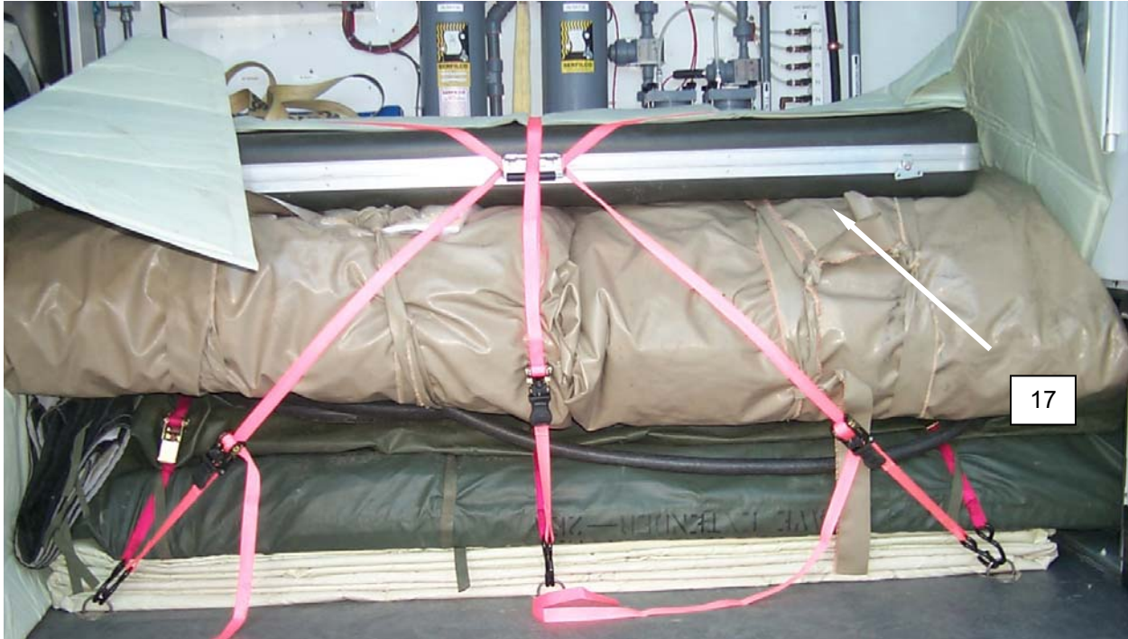
Figure 14. Placing the Light Case for Full Packout.
