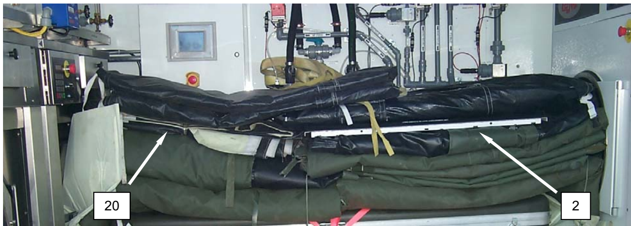
Figure 17. Placing the Inner Liner Fabric Sections.
