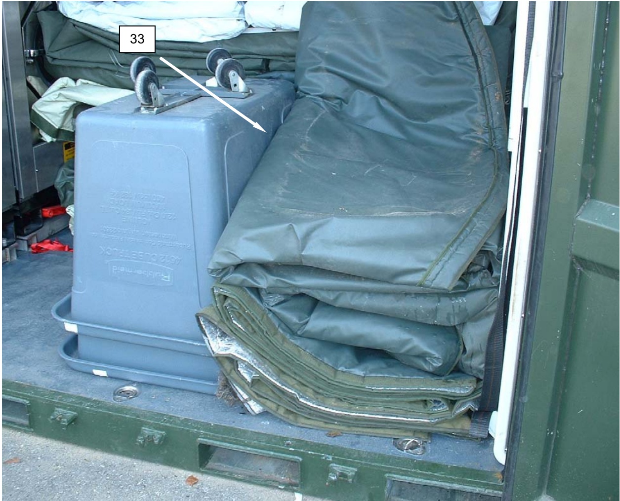
Figure 29. Place One Set of Water Tank Insulation.
