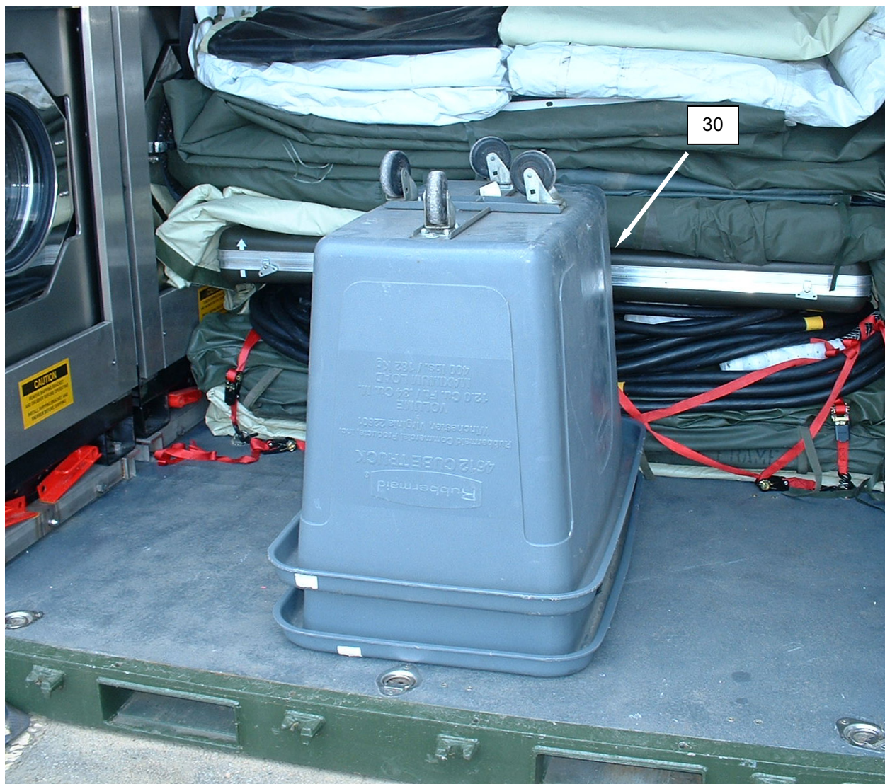
Figure 26. Both Inverted Laundry Bins over Inverted Trash Can.
