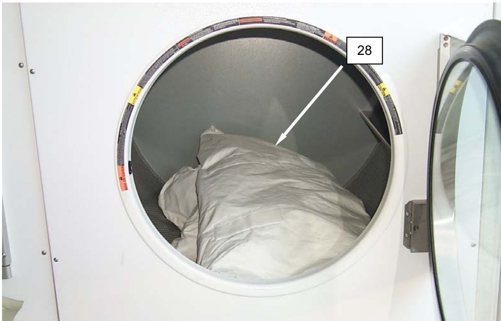
Figure 24. Folded TEMPER Plenum inside Dryer No. 2.
