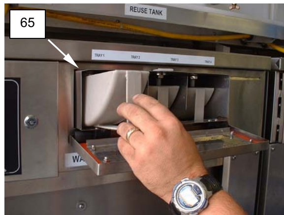
Figure 32. Add Antifreeze - Washer No. 1.
