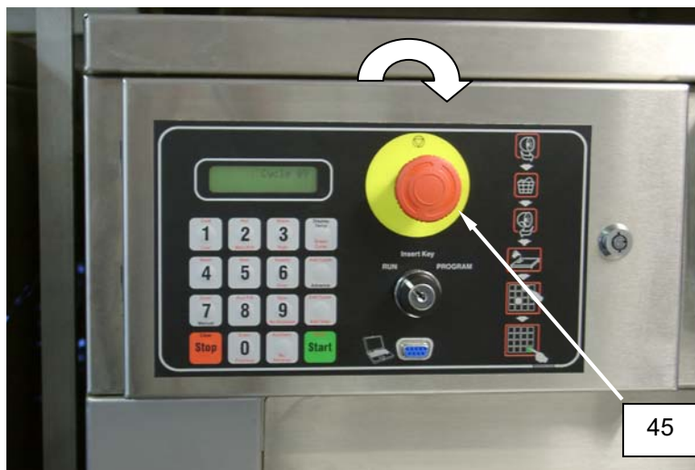
Figure 23. Emergency Stop Settings.
