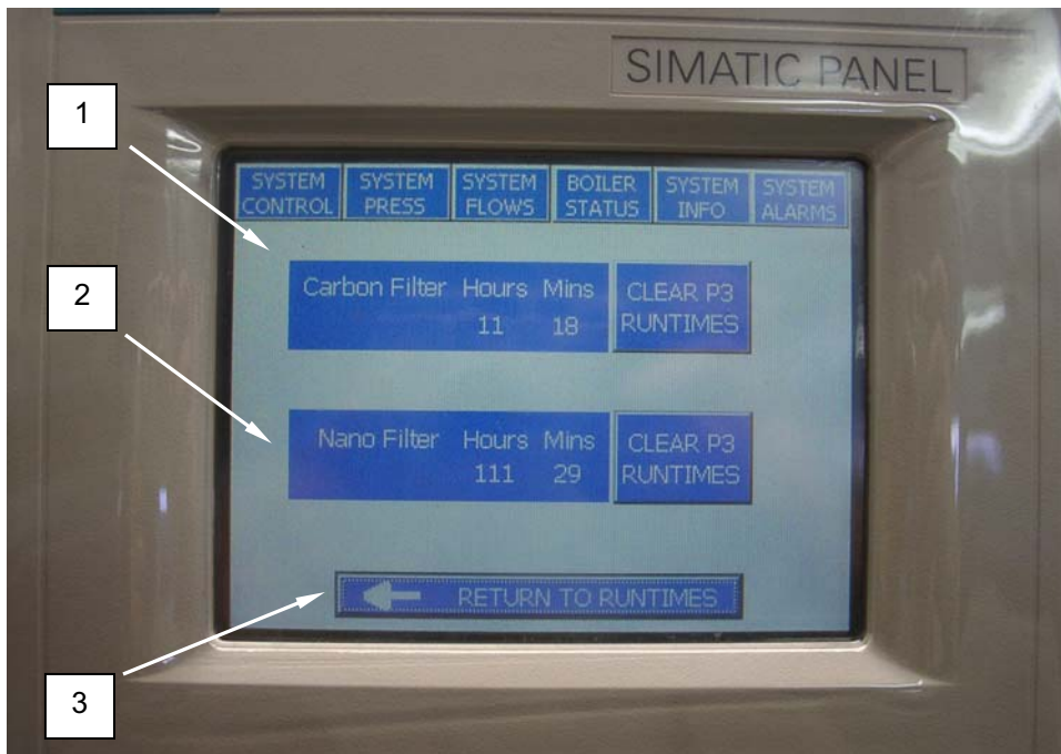
Figure 12. Additional Runtimes Display.
