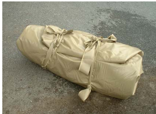
Figure 11. Prepare the 3000 Supply Water Tank for Movement.
