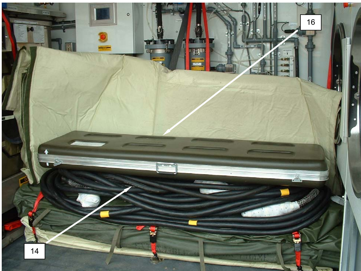
Figure 13. TEMPER light case on top of power cables.
