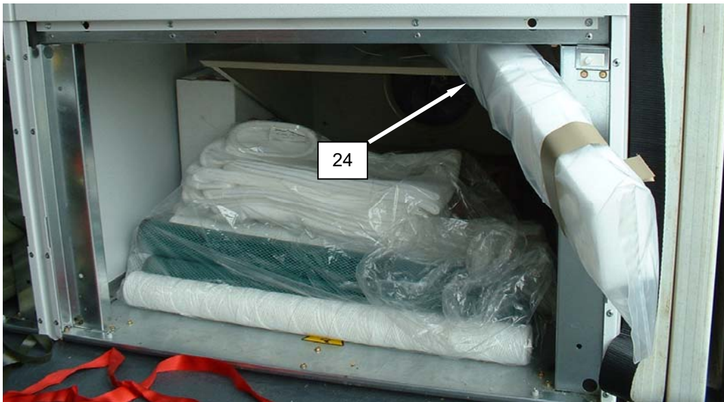
Figure 19. Placing the Water Tank Floats for Full Packout.
