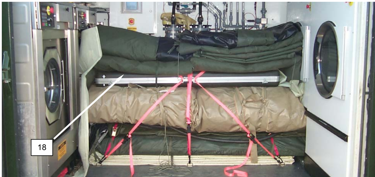
Figure 16. Placing the Fabric Sections.
