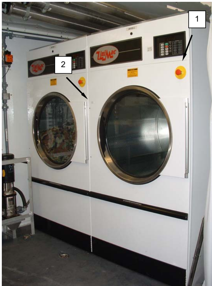
Figure 3. Door Open Indicator.
